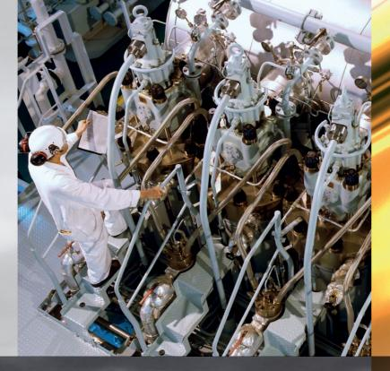
**YOUR OPERATING ENVIRONMENT** is tough which can compromise engine performance. Highly rated and efficient modern engines commonly operate with low oil consumption and small specific sump capacities. Fuel contamination is a common side effect of high pressure injection and **heavy fuel oils** may have variable sulphur content which can lead to engine problems.
